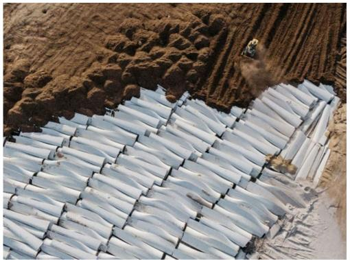
Turbine blade cemetery - a yellow bulldozer buries used wind turbine blades..
